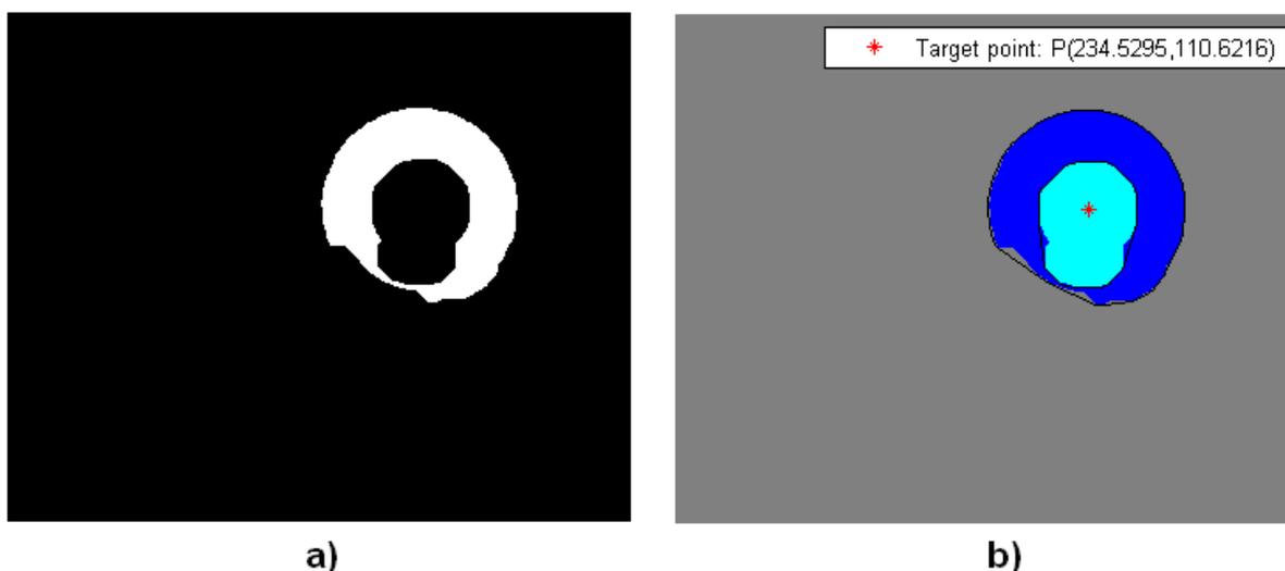
Figure 11. a) Unexpected binary image; b) incorrect region extraction.
