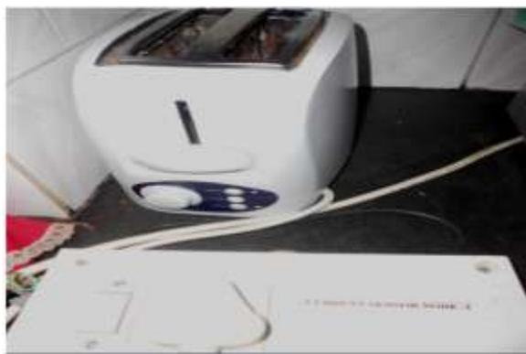
Figure 4. Current sensor node connected to a toaster in kitchen.
