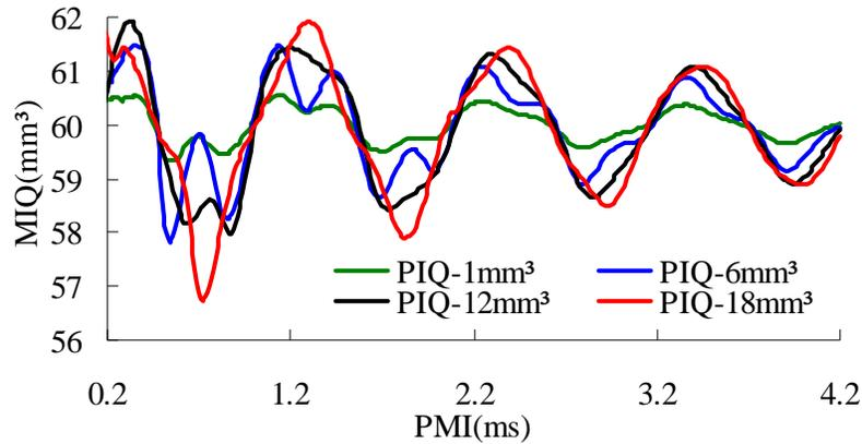
Figure 7. MIQ with different PIQ in pilot-main injection
