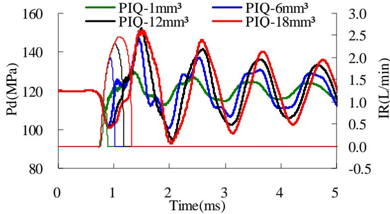
Figure 8. Delivery chamber pressure and injection rate with different PIQ and no main injection
