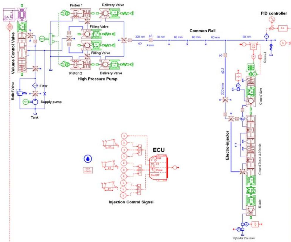
Figure 3. AMESim simulation model of the HPCR system
