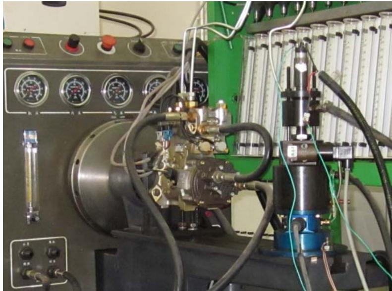
Figure 4. Experiment test bench of HPCR system
