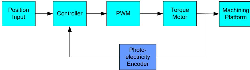
Figure 1. The structure of servo feed system based on a Photo–electricity Encoder
