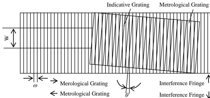
Figure 3. The schematic of grating measurement
