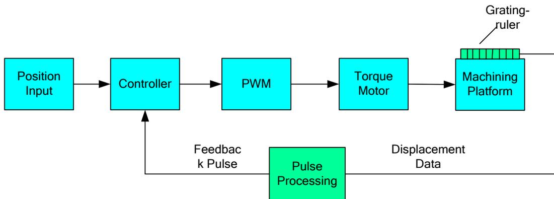
Figure 2. The experimental set-up diagram of servo feed system based on a grating ruler
