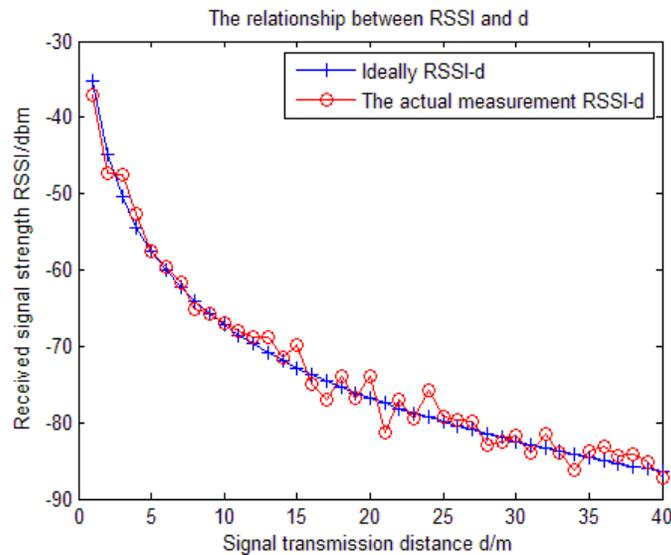
Figure 2. The relationship between RSSI and signal transmission distance
