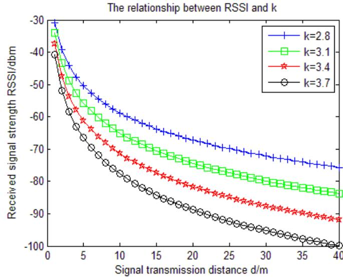
Figure 1. The relationship between RSSI and path loss factor
