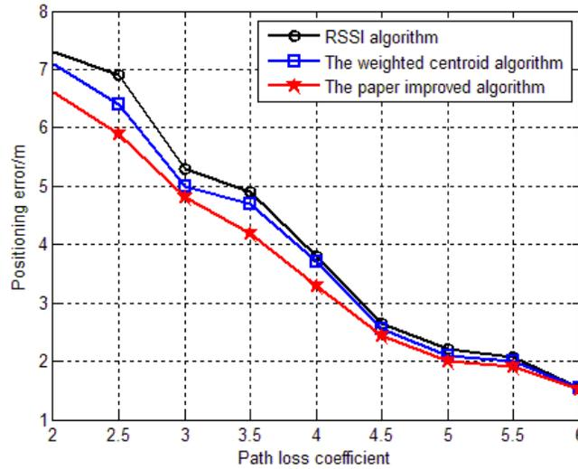
Figure 8. Effect of path loss coefficient of positioning error
