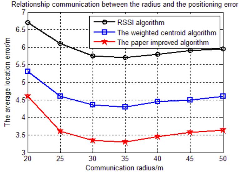
Figure 10. Impact of node communication radius of positioning error
