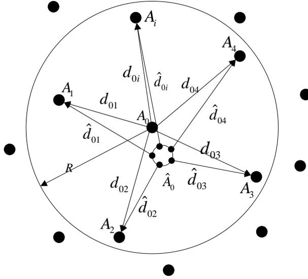
Figure 4. Differential correction positioning of beacon node
