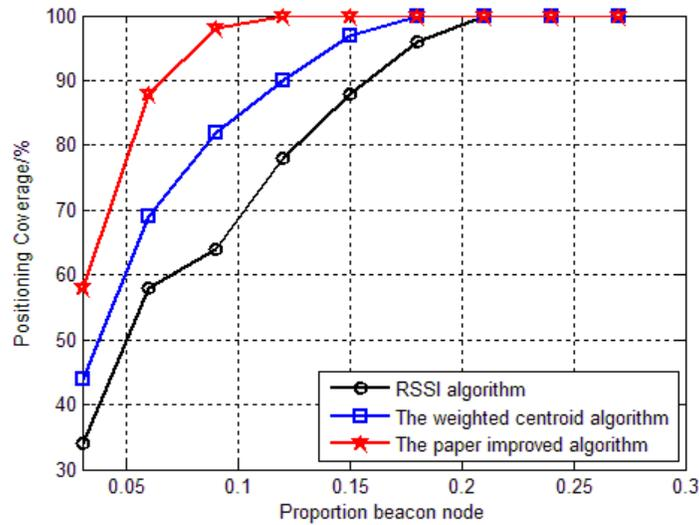
Figure 7. The relationship between the percentage of beacon nodes and the coverage rate of positioning
