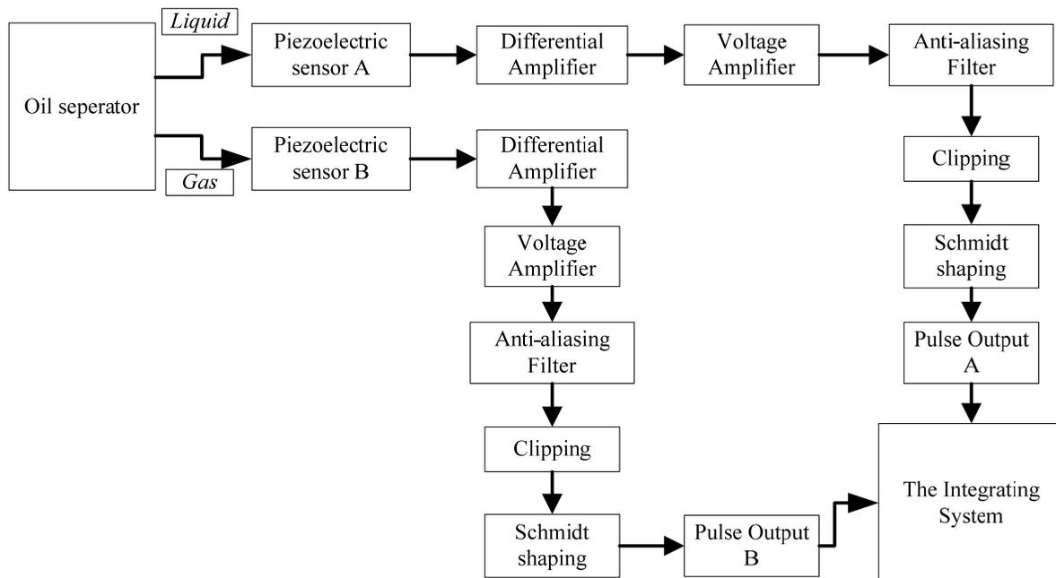
Figure 3. The block diagram about signal conditioning
