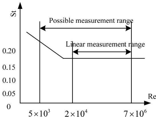
Figure 2. The graph of *St*'s measurement range
