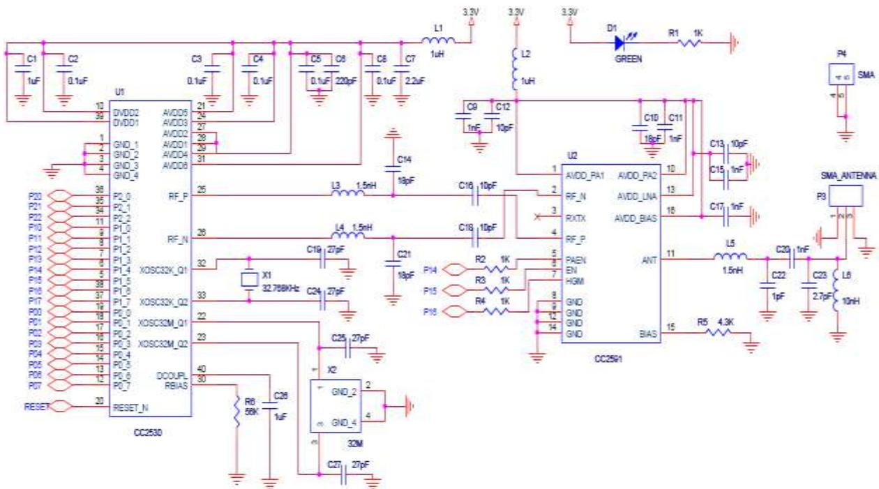
Figure 5. The circuit of the CC2530 Zigbee node
