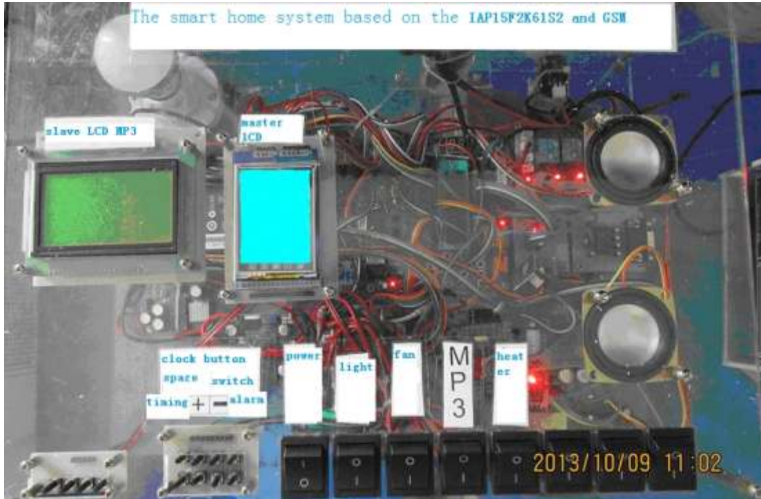
Figure 10. The smart home system based on the IAP15F2K61S2 and GSM
