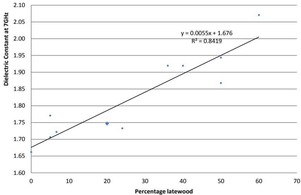
Figure 5. Measured Dielectric constant at 7GHz versus percentage late wood in the sample
