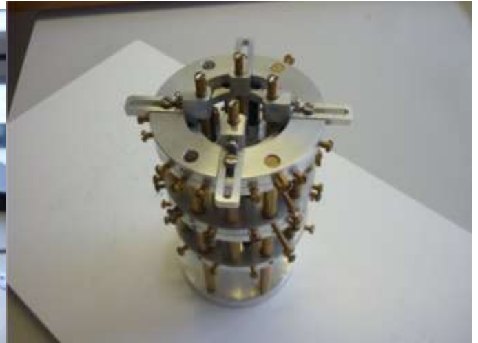
(b) Halbach prototype with the slide-blocks used to move the shim magnets in radial direction.
