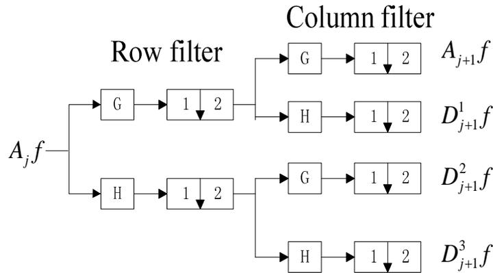
Figure 4. (a)Mattiat Two dimensional wavelet decomposition algorithm
