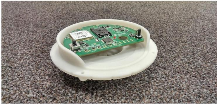
Figure 5. System Enclosure, lower half with PCB placed
