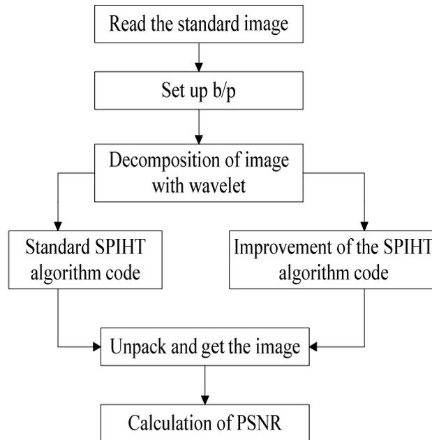
Figure 4. The flow chart of software implementation.
