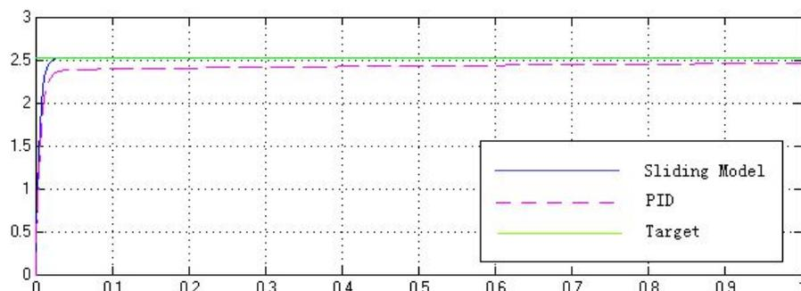
Figure 5. The comparison of tracking current of step power-assisted motors in different algorithms
