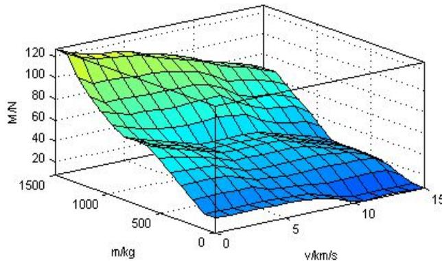
Figure 2. The three dimensional graph of the biggest power-assisted steering torque
