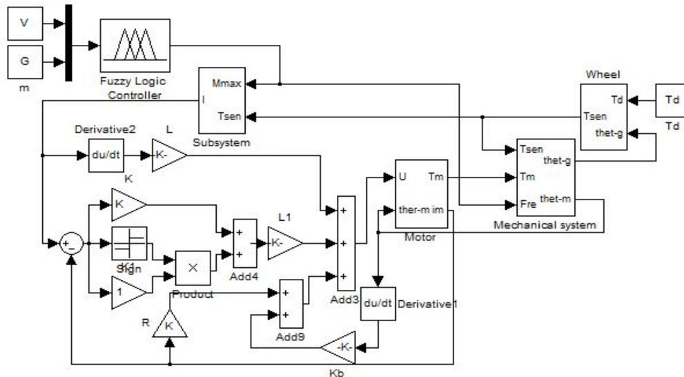
Figure 4. The simulation model diagram of forklift EPS system using SMVSC
