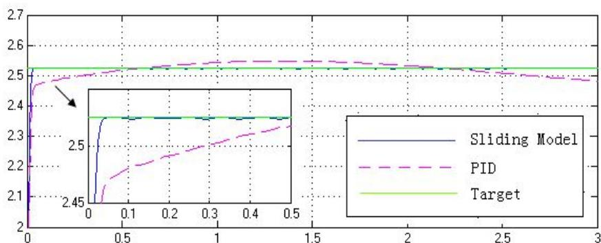
Figure 7. The simulation of tracking current of step power-assisted motors in different algorithms when disturbed
