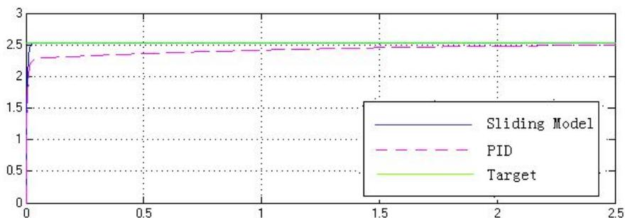
Figure 6. The comparison of tracking current of step power-assisted motors in different algorithms when changing parameters
