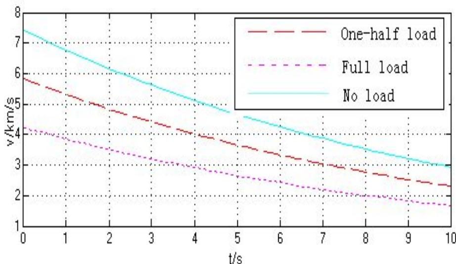
Figure 10. The safety speed changing curve under different steering conditions
