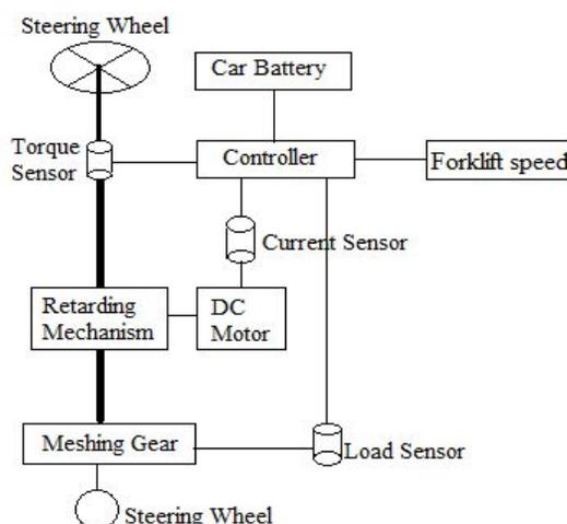
Figure 1. Forklift EPS system structure diagram
