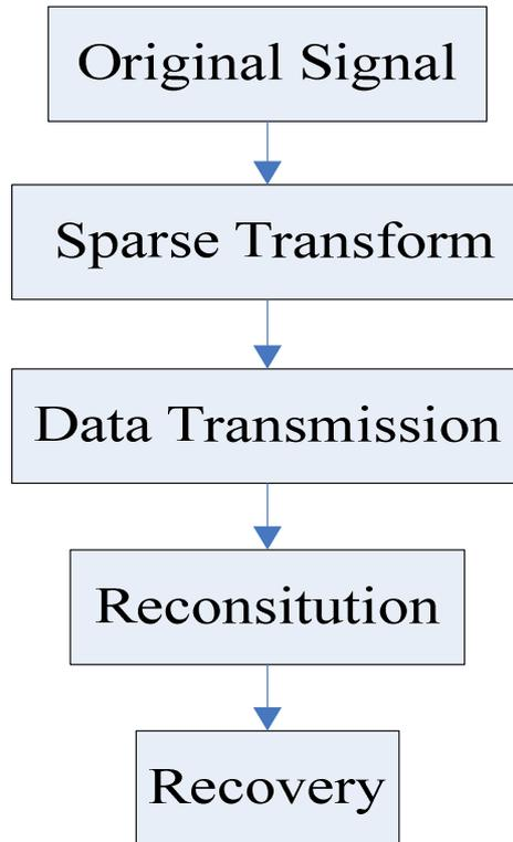
Figure 1. The framework of compressed sensing.
