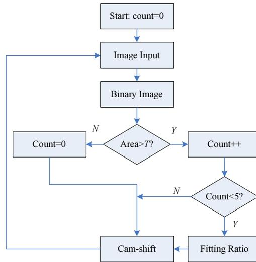
Figure 5. The flowchart of Cam-shfit algorithm
