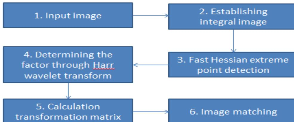
Figure 7: The basic framework of SURF
