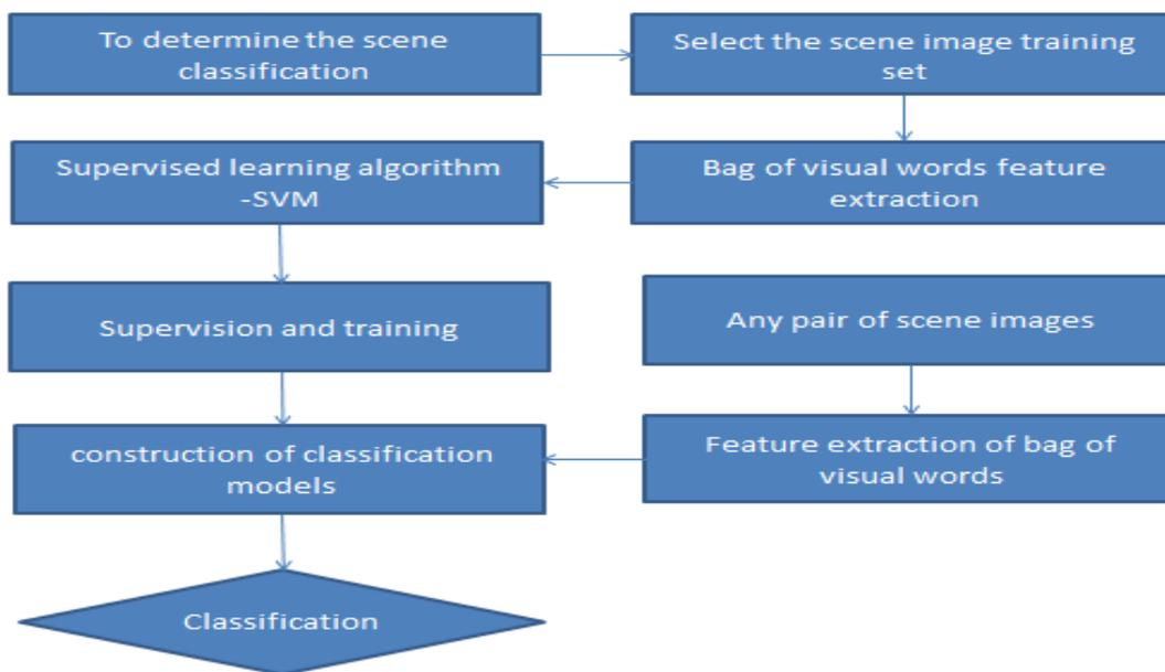
Figure 8: SVM Image classification system based on the bag of words model
