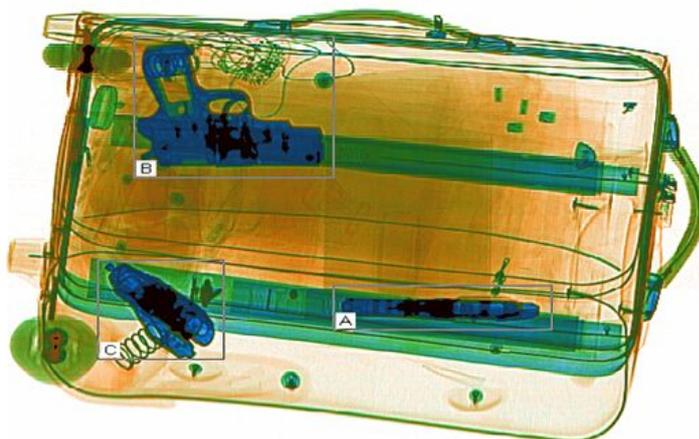
Figure 1: X-ray machine image of the same pistol in the same case from three different placing angles
