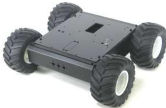
Figure 3. Robot skid-steering Rover 4WD1
