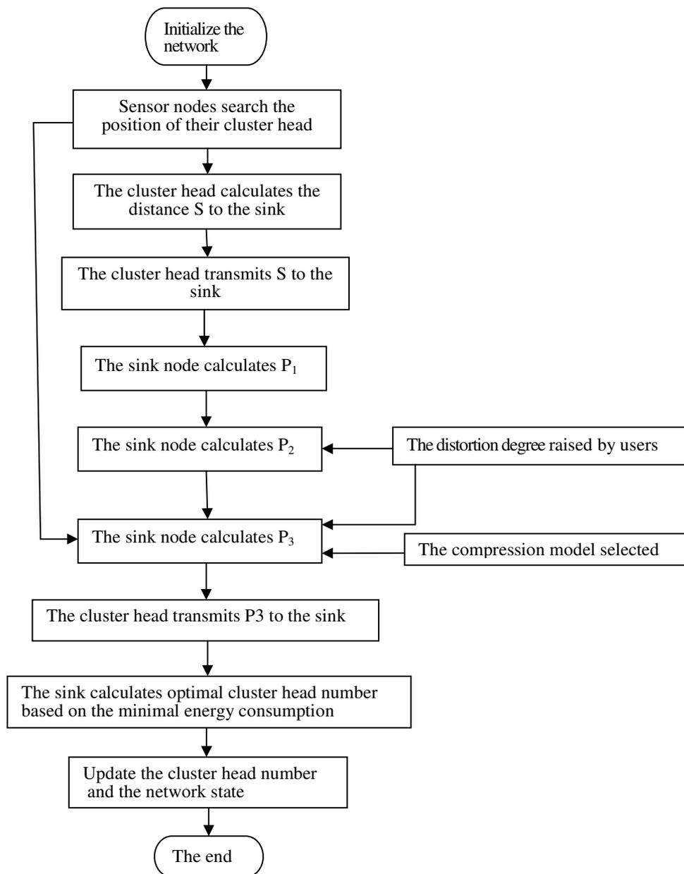
Figure 3. Process flow of OCHN
