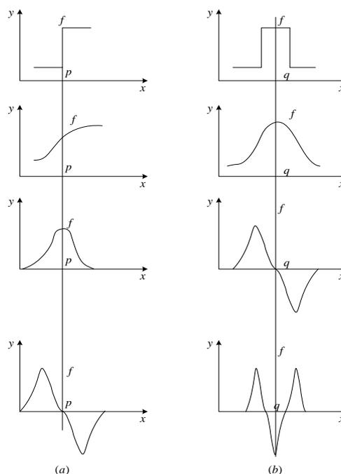
Figure 1 Sectional view of image edge, first derivative and second derivative
