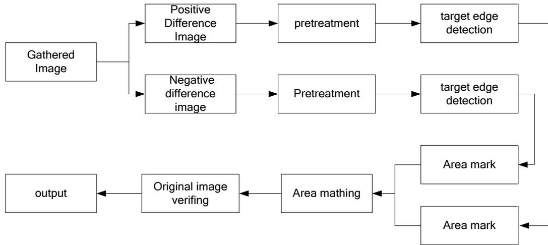
Figure 8 Processing algorithmic diagram figure of difference image
