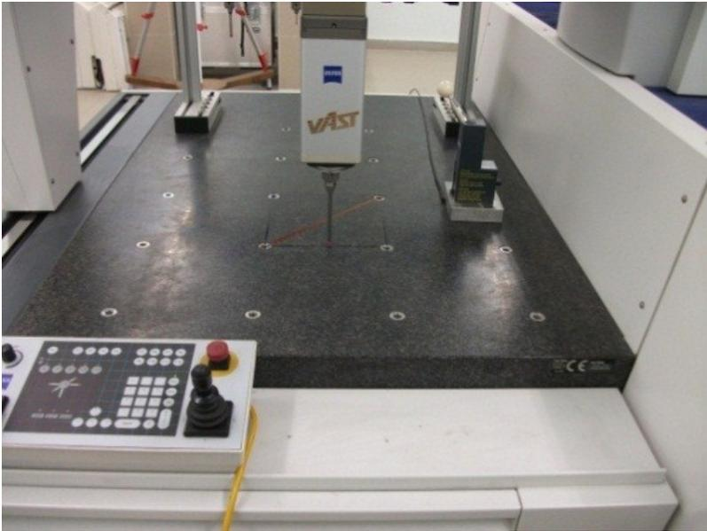
Figure 1. Straightness measurement in 2D using coordinate measuring machine
