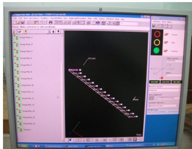
(a) An schematic of straightness 16 points distribution in X- direction
