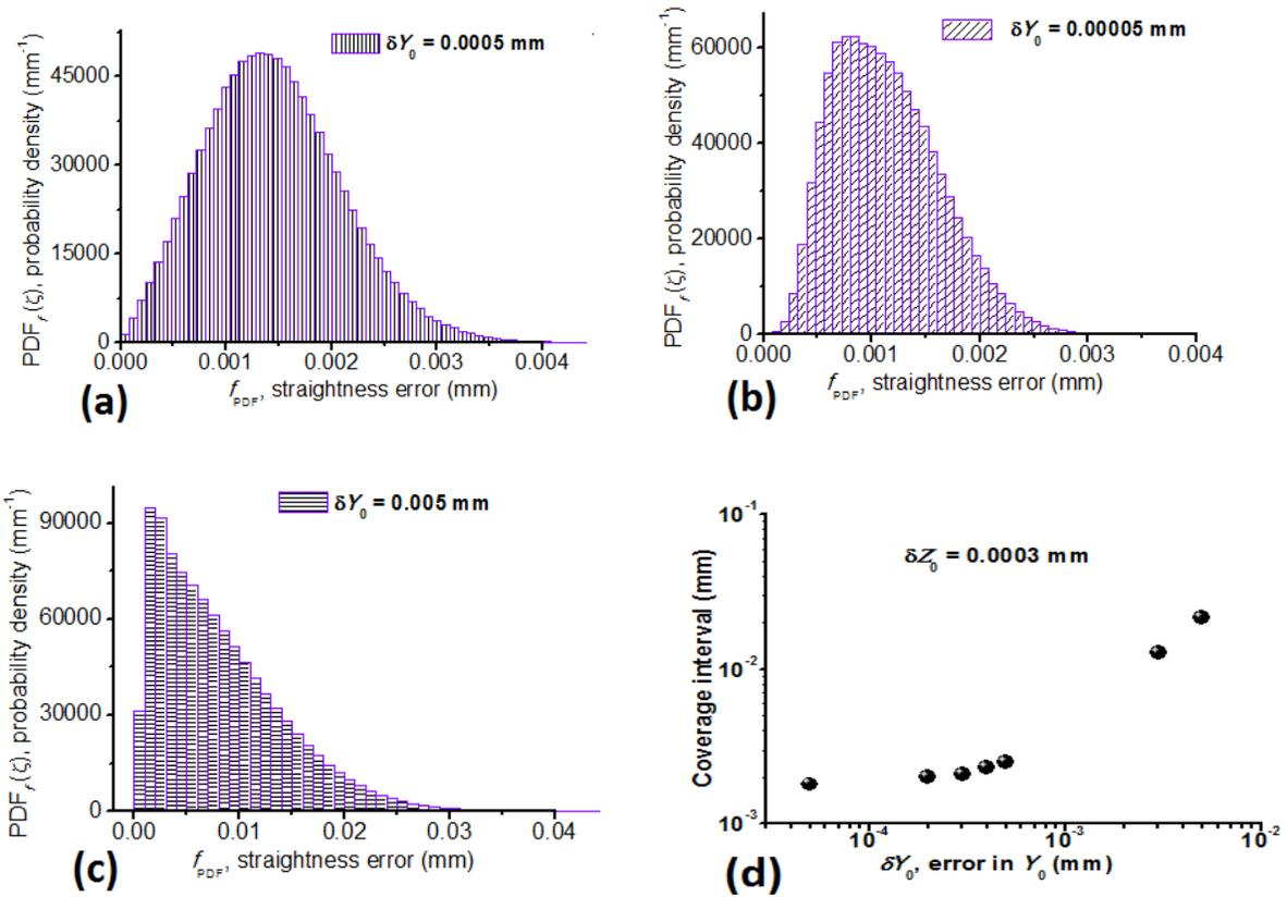
Figure 6. The probability density at  $\delta Z_0 = 0.0003 \text{ mm}$  as a function of the straightness error for (a)  $\delta Y_0 = 0.0005 \text{ mm}$  which is corresponding to error in the optimized  $\bar{Y}_0$  value in Table 2.
