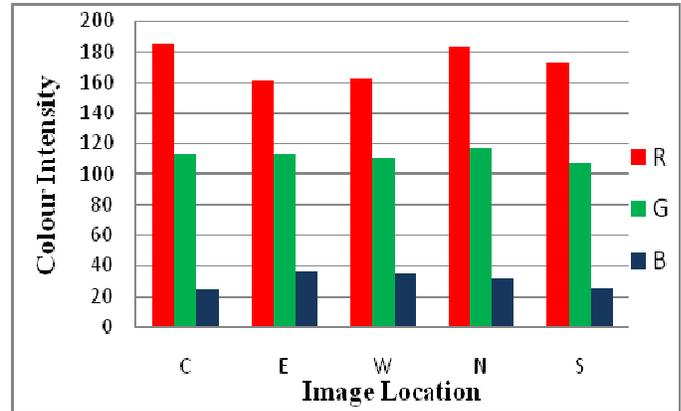
Fig.5 Average R, G, B intensity of the images at different locations in the sample holder (bowl)
