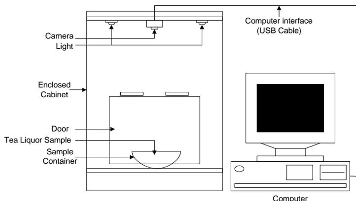
Fig. 2 Schematic diagram of Electronic Vision System
