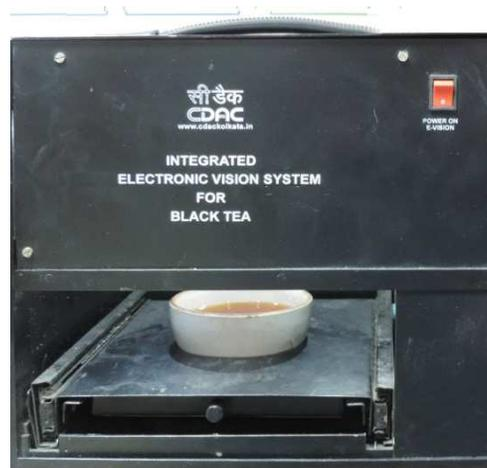
Fig. 3 Electronic Vision System (E-VISION)
