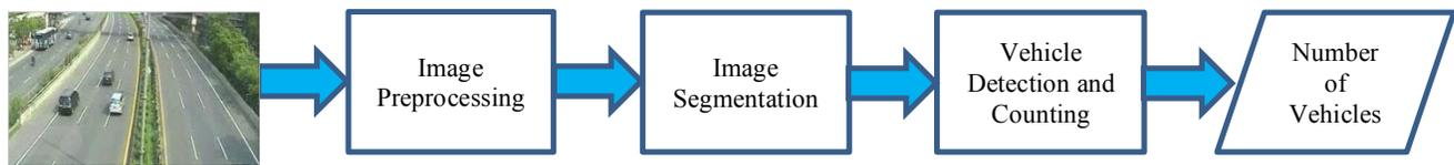
Figure 1. The Architecture of the Vehicle Detection and Counting System
