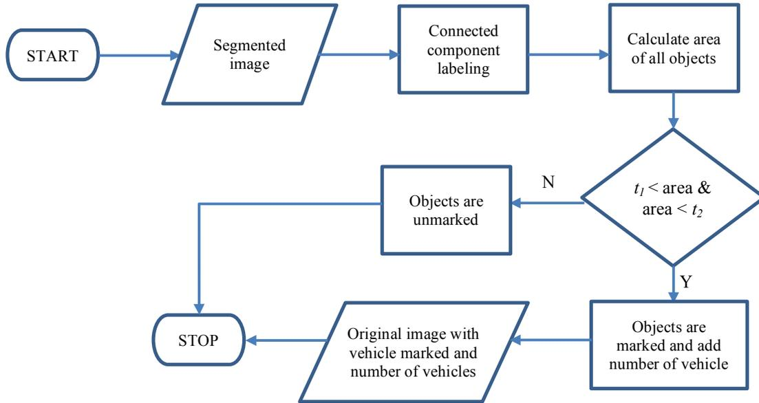
Figure 4. Counting Number of Vehicles Flow Diagram
