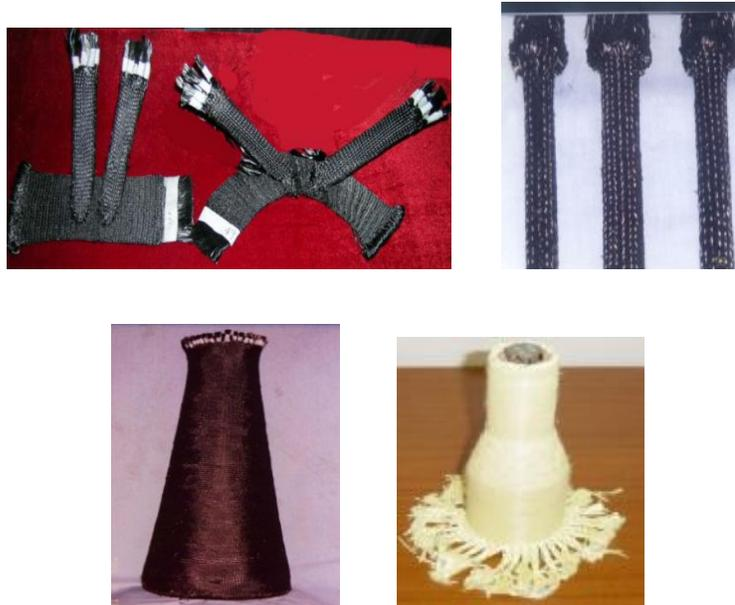
Figure 4. Drawing for Finished Product of 3-D Braided Composites.
