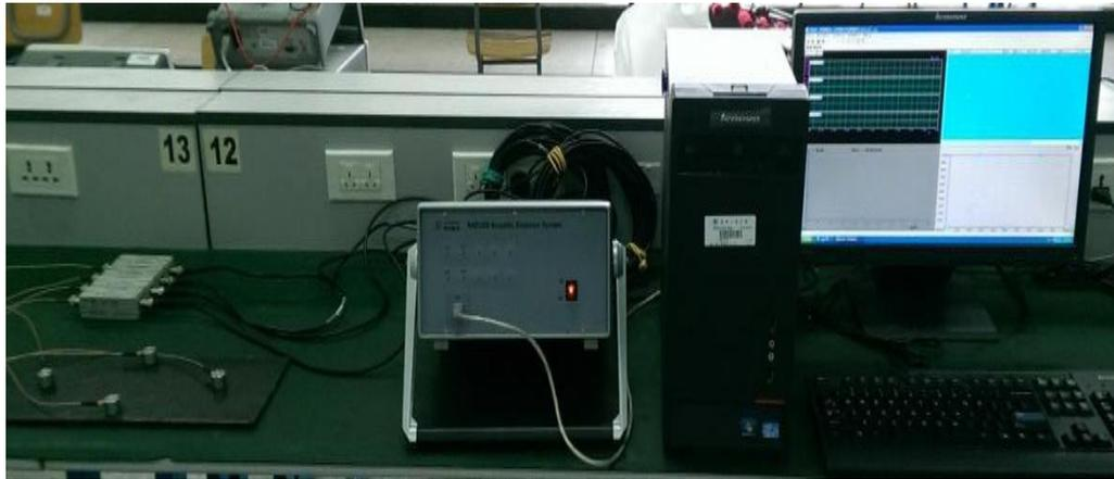
Figure 7. SAEU2S Acoustic Emission System
