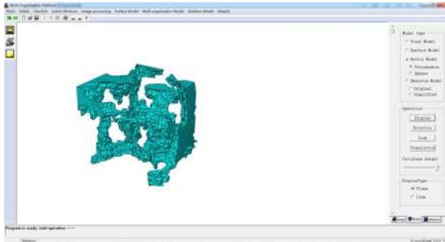
Figure 7. The visualization of complete three-dimensional solid model of carbonate rock core
