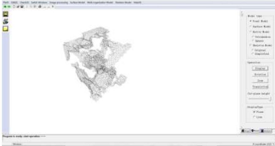
Figure 4. The visualization of three-dimensional voxel model of carbonate rock core
