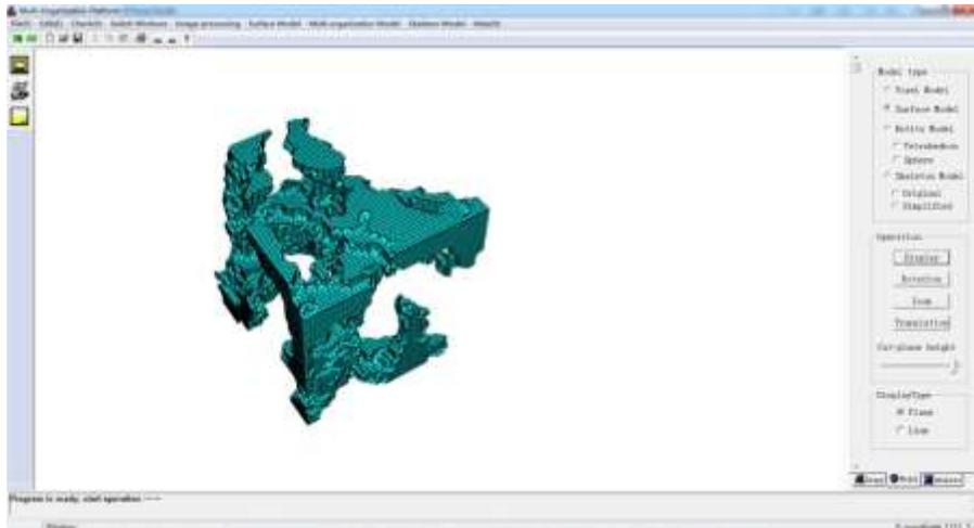
Figure 5. The visualization of complete three-dimensional surface model of carbonate rock core
