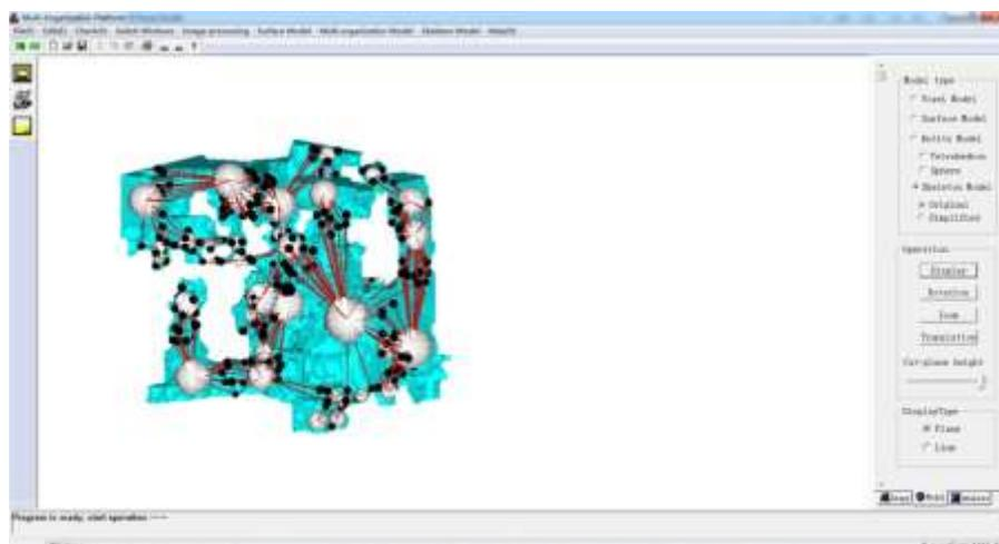
Figure 9. The visualization of complete three-dimensional skeleton model of carbonate rock core
