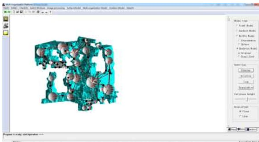
Figure 10. The visualization of sectional three-dimensional skeleton model of carbonate rock core
