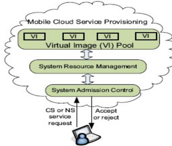
Fig. 2. Reference Model of Mobile Cloud Computing.
