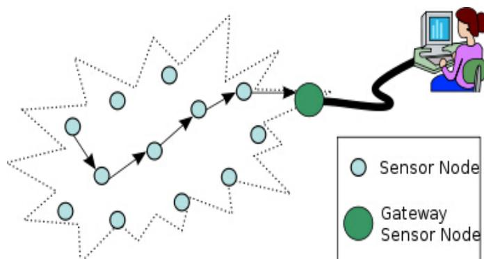
Figure 9. Typical multi-hop wireless sensor network architecture
