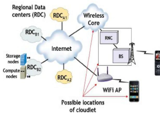
Fig. 1 Mobile Cloud Computing (MCC) architecture.
