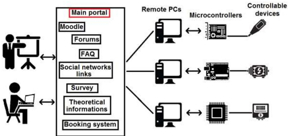
Figure 3. High-level Architecture of Our Remote lab System
