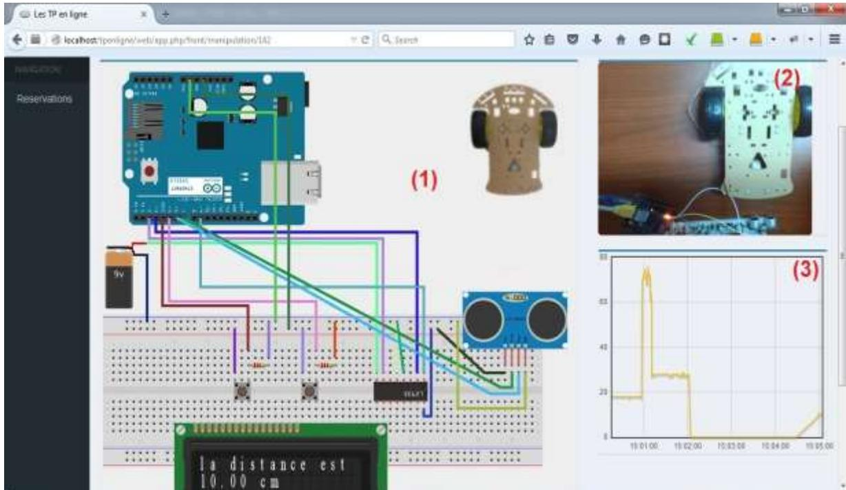
Figure 8. The remote laboratory manipulation page for practical work
