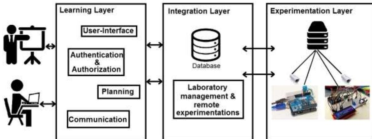
Figure 5. The three layers architecture of the remote laboratory
