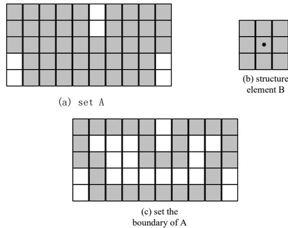
Figure 4. Boundary extraction diagram
