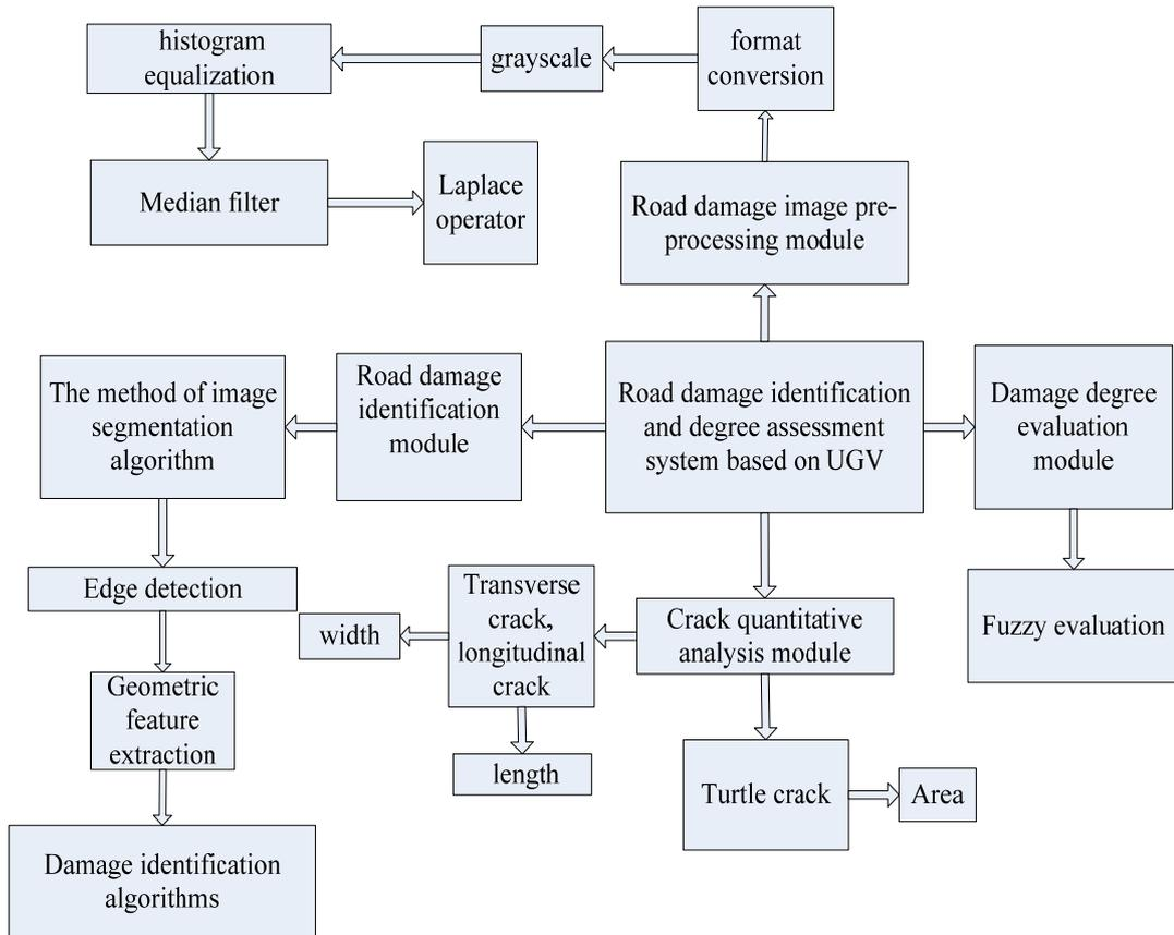
Figure 6. Function modules of the road damage degree recognition and assessment system
