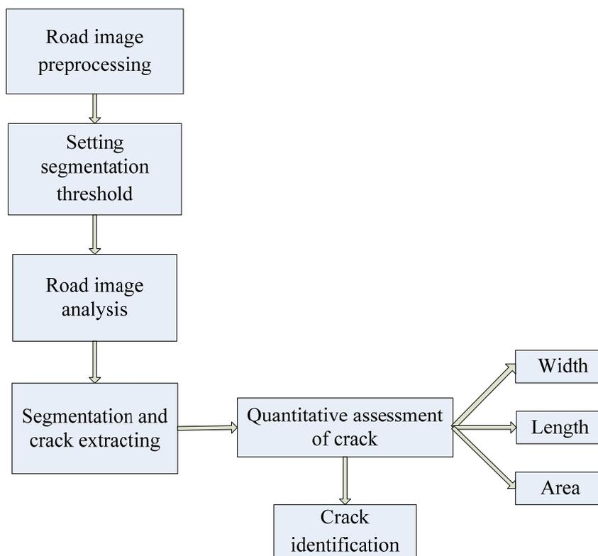
Figure 1. The processing algorithm of road crack image
